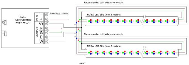
The installed power of the LED strips must be in accordance with the controller.
